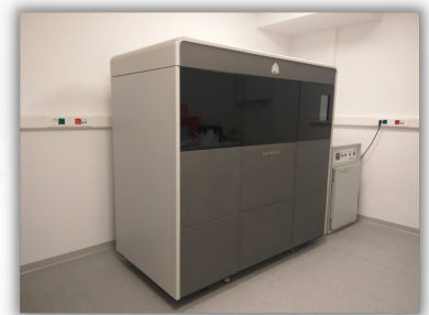
MJP5600 3D SYSTEMS LARGE FORMAT, MULTI MATERIAL COMPOSITE PARTS IN A SINGLE BUILD
